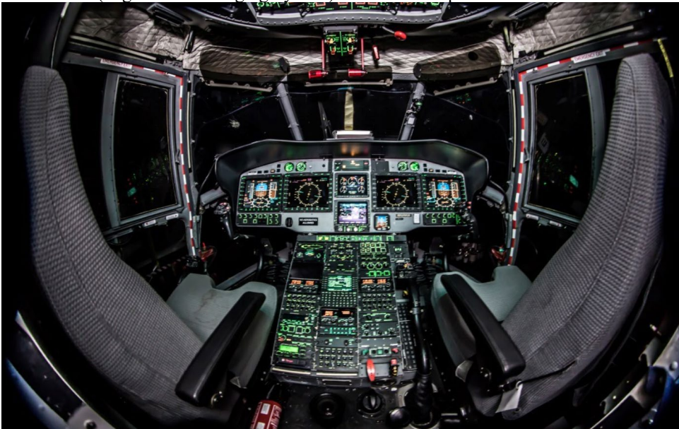
H225 NVIS (Night Vision Imaging System) modified cockpit. Photo courtesy of Global Helicopter Service
